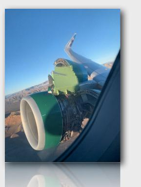
The airline reported the engine cowling came loose and separated from the aircraft.
