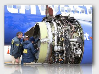
patterns from the fan blades on the engine from Flight 1380, the initial cracks were present during the 2012 inspection, but because the blades were inspected visually using fluorescent dyes to highlight flaws, they were missed by the inspectors. At that time, inspectors were not required to use ultrasound or other advance technology to detect such issues.
